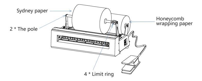
3, Start the machine to step on the foot switch once, and then put the paper close to the drum, the drum will automatically inhale the paper, and then step on the foot switch drum will stop sending paper and cut the paper once.
