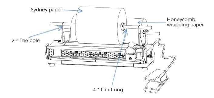
3. Send the appropriate paper length according to the items to be wrapped. After the package is finished, hold the black rubber wood handle ball in the manual paper cutting device and push it in the direction of the paper. (When cutting the paper, you should hold the handle ball with one hand and cut the paper, and the other hand slightly pull the wrapped items to make tension on the surface of the paper.)
